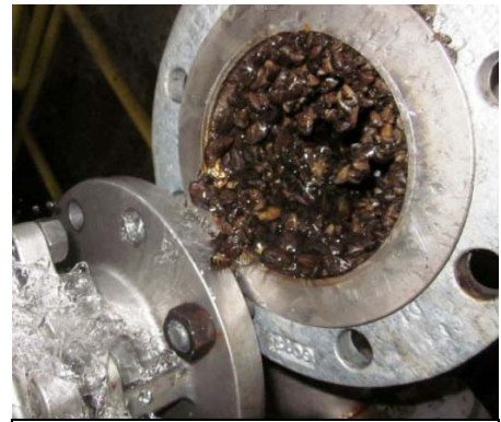
Mussels can clog a 4 inch pipe so no water can get through it.
