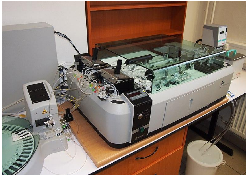
AutoAnalyzers measure the amount of nutrients in a water sample. PC: Wikimedia Commons (CC BY-SA 4.0)
