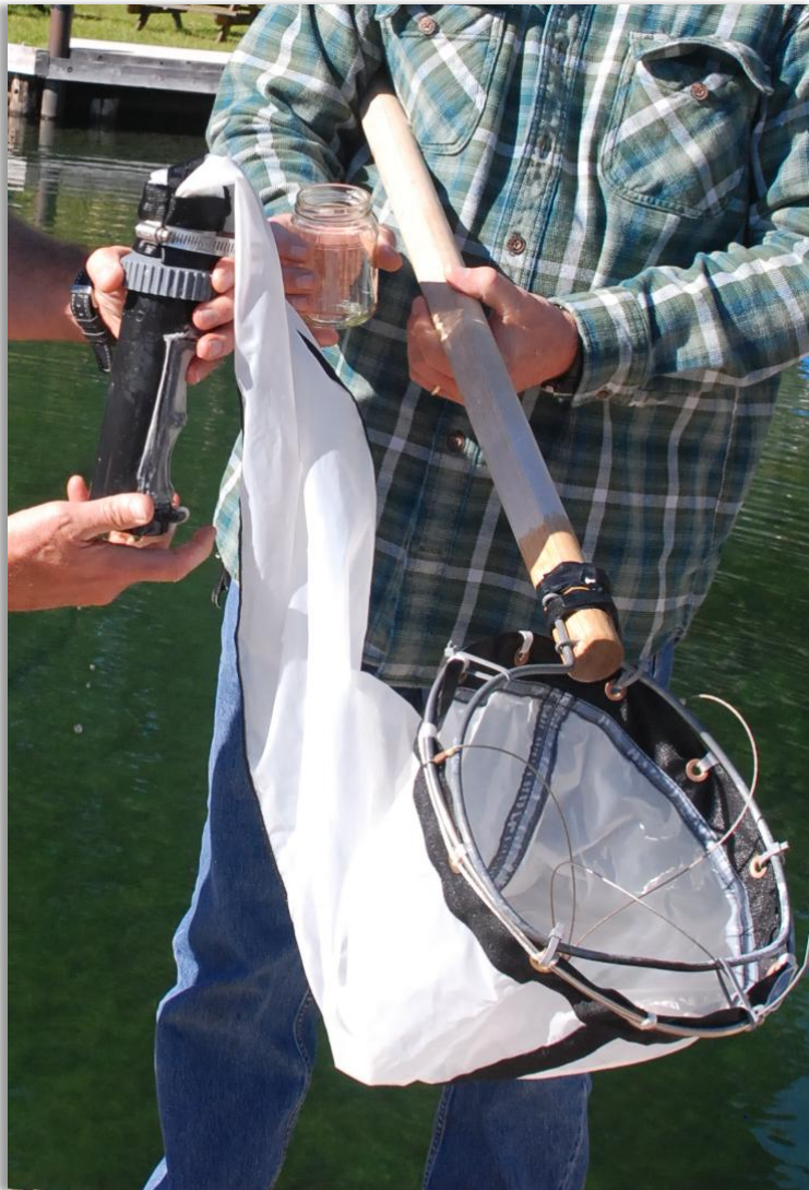
A zooplankton net. PC: Flathead Lake Biological Station
