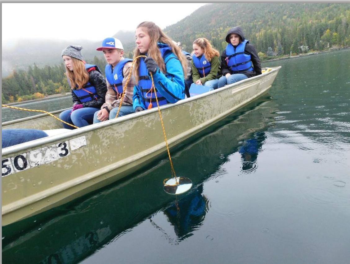
Measuring water transparency with a Secchi disk. PC: Flathead Lake Biological Station
