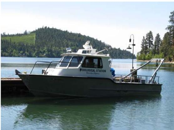
The *Jessie B*’s design still fulfills research requirements and the hull is in excellent condition, but the powertrain (engines, outdrives, propellers) and instrumentation need replacing and the hydraulic systems need rebuilding. It is also time for new windows, paint, trailer tires, etc.
