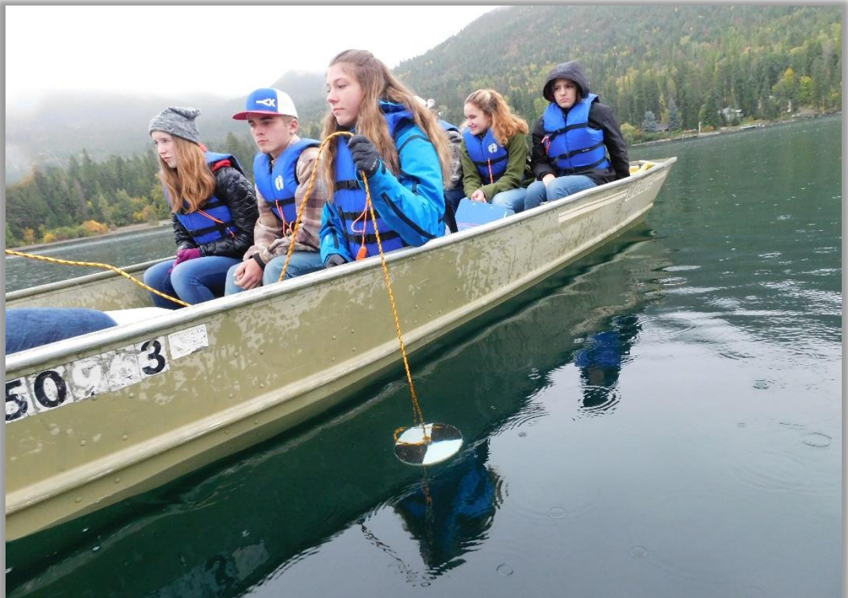
Measuring water transparency with a Secchi disk. PC: Flathead Lake Biological Station
