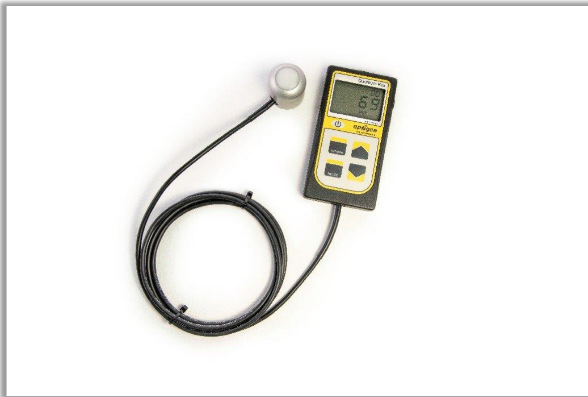
Underwater light meter used to measure water transparency. PC: DIYLED UK
