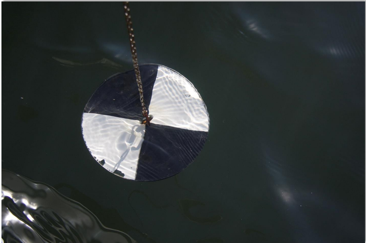
A Secchi disk is lowered into the water. PC: Minnesota Pollution Control Agency (CC BY-NC 2.0)
