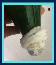
With a rubber band, secure a piece of cut cheese cloth around the opening of the water bottles. Make sure the cheese cloth has two layers to be strong enough to hold gravel and sand.
