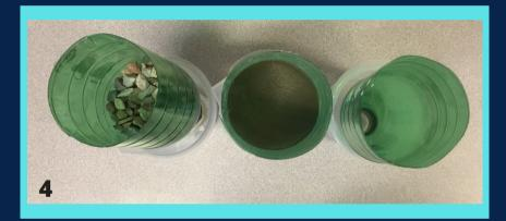
Add 3/4 cup of sand to one bottle, 3/4 cup of gravel to another, and leave the third water bottle empty. Place all 3 water bottles upsidedown into the plastic cups. Pour equal amounts of dirty water into the water bottles.
