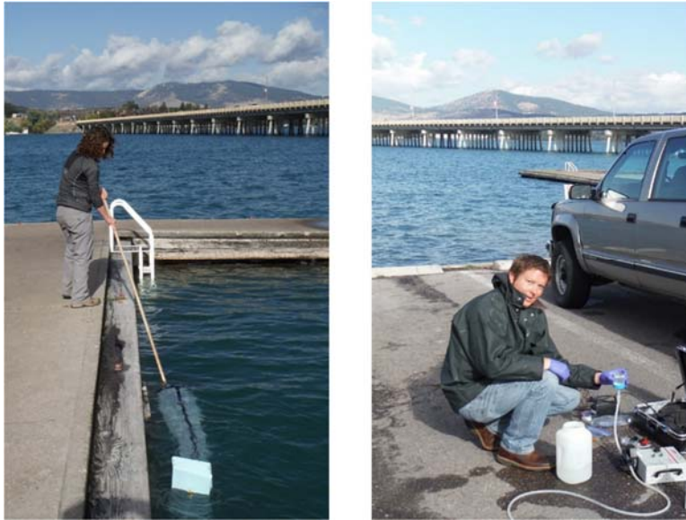
Figure.1. Environmental DNA sample collection by plankton tow net (left) and by filter (right)
